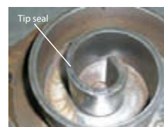
Melted tip seal; scored scroll spiral
