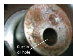
Inner surface of oil hole is plated by rust
