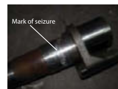
Bearing seized as oil film destroyed by water
