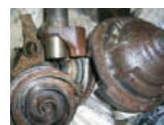
Mechanical parts and shell are rusty
