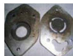
Carbonized valves and valve plates
