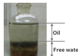
Free water in oil (Evaporator leak)
